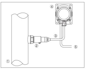
Fig. 15: Configuration, process module, external housing
