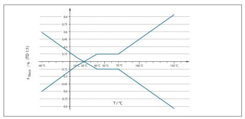
Fig. 33: Basic temperature error F<sub>TBasis</sub> at TD 1 : 1
