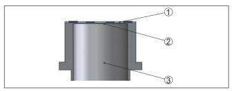
Fig. 4: Configuration of the measuring system with strain gauge (DMS) sensor element
