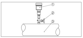
Fig. 11: Measurement setup for process pressure measurement of gases in pipelines
