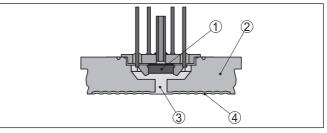
Fig. 3: Configuration of the measuring system with piezoresistive sensor element
