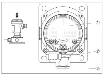
Fig. 22: Electronics and connection compartment
