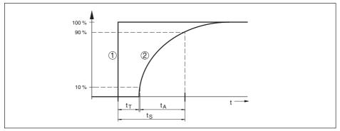
Fig. 32: Behaviour in case of sudden change of the process variable.  $t_{\tau}$  dead time;  $t_{s}$ : rise time;  $t_{s}$ : jump response time
