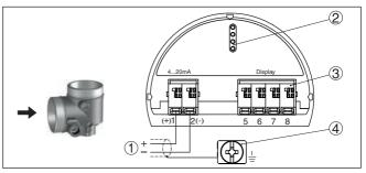
Fig. 19: Connection compartment - double chamber housing
