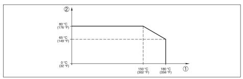
Fig. 39: Temperature derating IPT-2x, version up to +180 °C (+356 °F)
