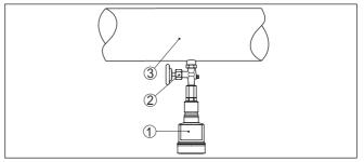
Fig. 13: Measurement setup for the process pressure measurement of liquids in pipelines
