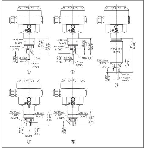
Fig. 49: IPT-2x, threaded fitting not front-flush
