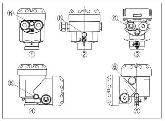
Fig. 7: Position of the filter element
