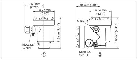
Fig. 42: Housing versions in protection IP66/IP67 (with integrated display and adjustment module the housing is 9 mm/0.35 in higher)
