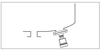
Fig. 14: Measurement setup for the level measurement
