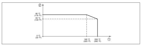
Fig. 40: Temperature derating IPT-2x, version up to +200 °C (+392 °F)
