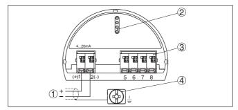
Fig. 24: Electronics and connection compartment - single chamber housing
