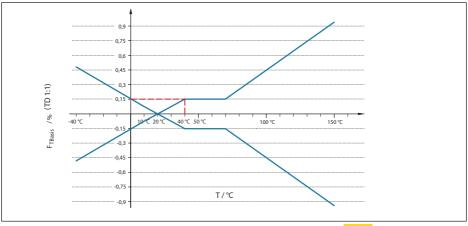
Fig. 41: Determination of the basic temperature error for the above example:  $F_{TBasis} = \frac{0.15 \%}{0.15 \%}$
