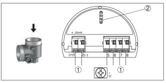
Fig. 18: Electronics compartment - double chamber housing
