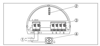
Fig. 17: Electronics and connection compartment - single chamber housing
