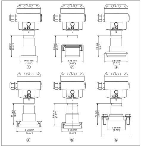
Fig. 52: IPT-2x, hygienic fitting 150 °C (metallic/ceramic measuring cell)
