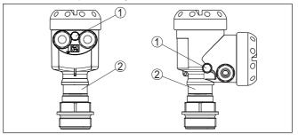
Fig. 9: Position of the filter element - gastight leadthrough
