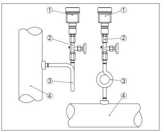
Fig. 12: Measurement setup for the process pressure measurement of gases in pipelines
