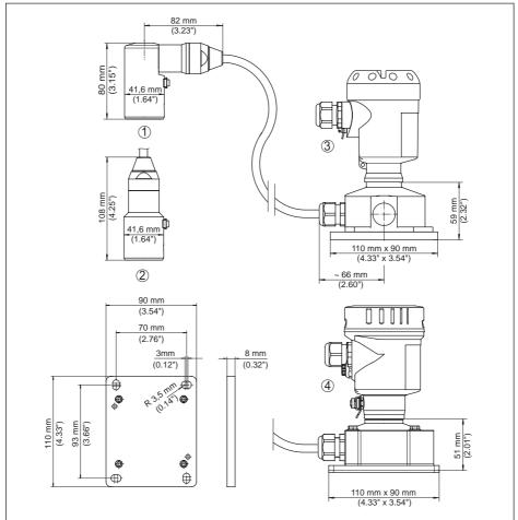
Fig. 48: IP68 (25 bar) version with external housing
