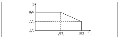
Fig. 37: Temperature derating IPT-2x, version up to +150 °C (+302 °F)
