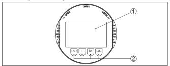
Fig. 27: Display and adjustment elements
