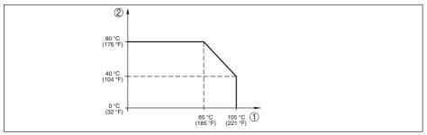
Fig. 36: Temperature derating IPT-2x, version up to +105 °C (+221 °F)
