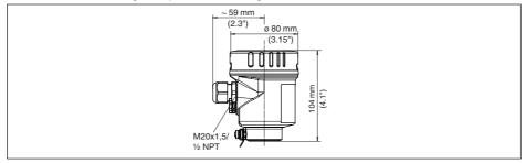
Fig. 47: Housing version with protection rating IP69K (with integrated display and adjustment module the housing is 9 mm/0.35 in higher)
