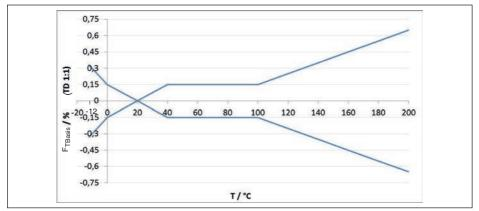
Fig. 34: Basic temperature error F<sub>TBasis</sub> at TD 1 : 1
