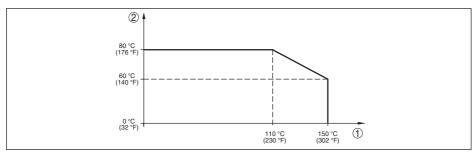
Fig. 38: Temperature derating IPT-2x, version up to +150 °C (+302 °F)
