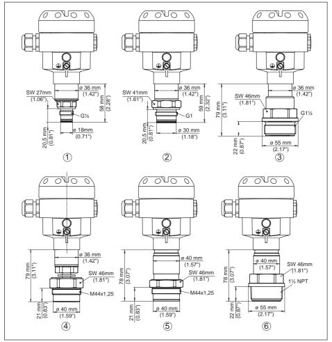
Fig. 50: IPT-2x, threaded fitting front-flush
