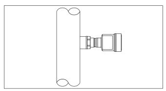
Fig. 2: Process pressure measurement IPT-2x
