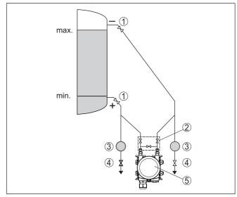
Fig. 13: Measurement setup, level measurement in closed vessel
