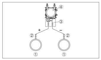
Fig. 20: Measurement setup with differential pressure measurement between two pipelines in gases and vapours
