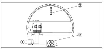
Fig. 31: Electronics and connection compartment - single chamber housing
