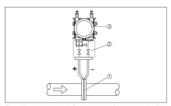
Fig. 17: Measurement setup with flow measurement of gases, connection via 3-fold valve block, flanging on both sides
