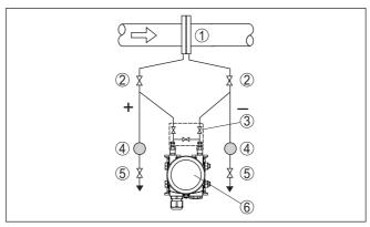
Fig. 19: Measurement setup, flow measurement in liquids
