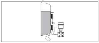
Fig. 5: Density measurement with DPT-20
