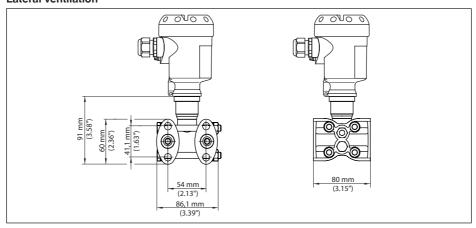
Fig. 46: DPT-20, 1/4-18 NPT connection, with lateral ventilation
