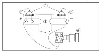
Fig. 23: Measurement setup, differential pressure measurement in gases, vapours and liquids
