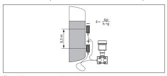
Fig. 24: Measurement setup for density measurement
