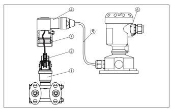
Fig. 40: DPT-20 in IP68 version, 25 bar and lateral cable outlet, external housing
