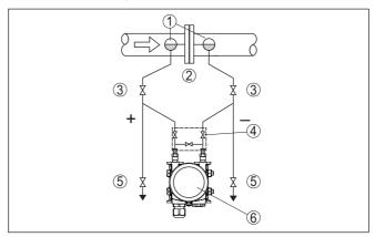
Fig. 18: Measurement setup, flow measurement in vapours
