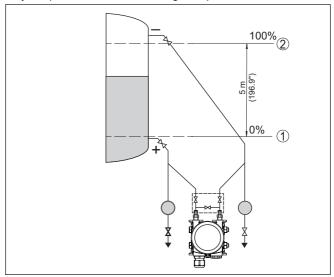
Fig. 34: Parameter adjustment example "Min./max. adjustment, level measurement"
