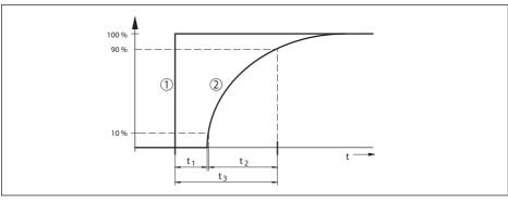
Fig. 41: Behaviour in case of sudden change of the process variable.  $t_i$ : dead time;  $t_2$ : rise time;  $t_3$ : jump response time
