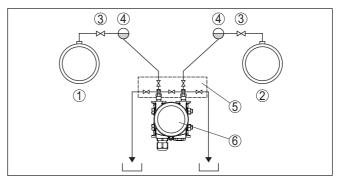
Fig. 21: Measurement setup with differential pressure measurement between a vapour and a condensate cable
