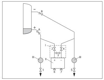
Fig. 35: Preferred measurement setup for closed vessels
