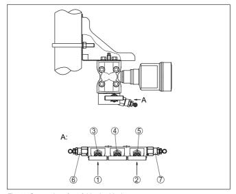
Fig. 12: Connection of a 5-fold valve block
