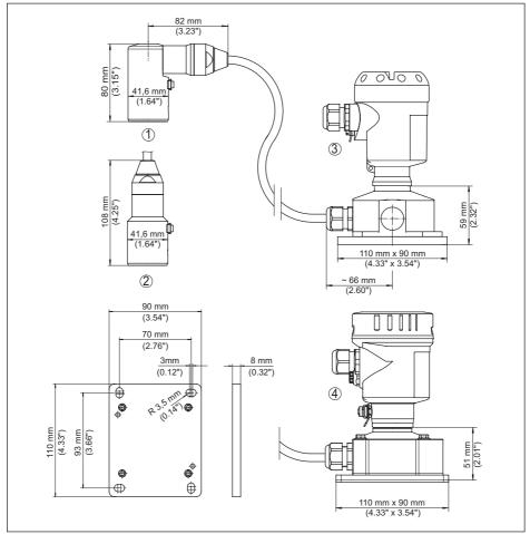
Fig. 44: IP68 version with external housing
