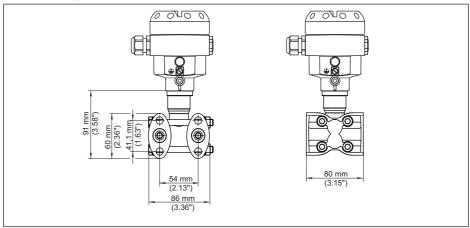
Fig. 45: DPT-20, ventilation on process axis
