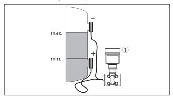
Fig. 15: Measurement setup, level measurement in closed vessel
