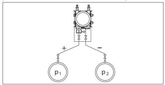
Fig. 4: Measurement of the differential pressure in pipelines with DPT-20, differential pressure  $\Delta p = p_1 - p_2$
