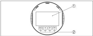
Fig. 33: Display and adjustment elements
