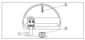
Fig. 27: Electronics and connection compartment - single chamber housing
