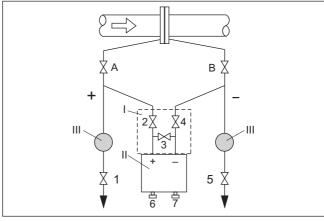
Fig. 38: Preferred measurement setup for liquids
