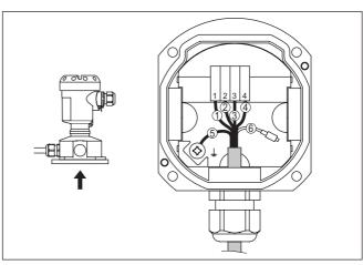
Fig. 30: Connection of the process component in the housing base
