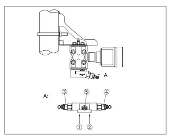
Fig. 10: Connection of a 3-fold valve block
