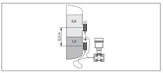
Fig. 25: Measurement setup with interface measurement
