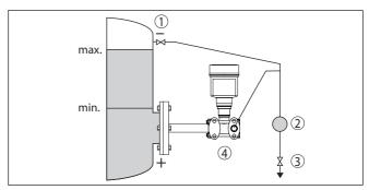
Fig. 14: Measurement setup, level measurement in closed vessel
