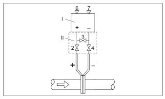
Fig. 37: Prefered measurement setup for gases, connection via 3-fold valve block, flanging on both sides
