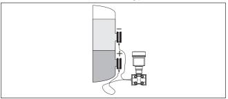
Fig. 6: Interface measurement with DPT-20
