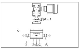
Fig. 11: Connection of a 3-fold valve block, flanging on both sides
