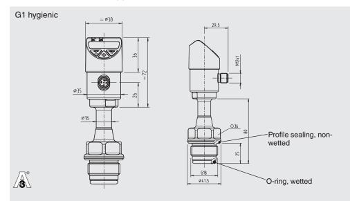
Suitable for WIKA adapter system model 910.61 For dimensions of the appropriate process adapters and welding sockets see data sheet AC 09.20
